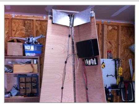
• The Arduino that reads the pots and controls the climbers is in the box on the back side, right above the 4D battery holder. Add some tape to the meeting point of the snow caps to keep the wires from snagging and to keep the snow caps from touching each other. Keep the back side of the game as neat as possible to avoid snags as the climbers climb.
